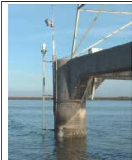
Figure 7: Stilling wells and air-acoustic tide gauges installed at four (4) locations, including:
